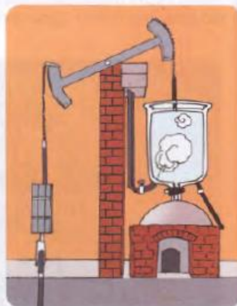
The first steam engine was used to pump water out of mines.
